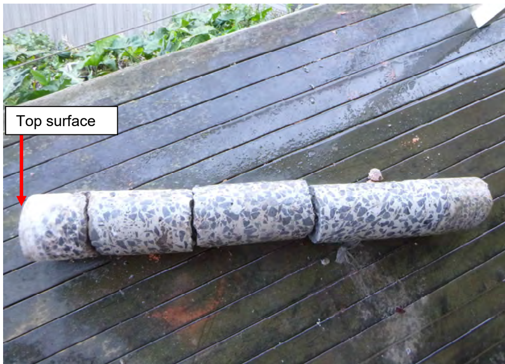
Photo D1 – View of concrete cored from beneath the balcony of Unit 2 (Borehole BH202). The start / top of the core is indicated as shown.
