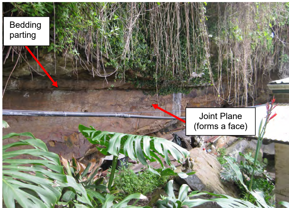
Mapping Traverse 102, Photo 5 – View of overhang in cross-bedded sandstone to the north of traverse 102. Continuous bedding plane and undulating joint plane indicated as shown.
