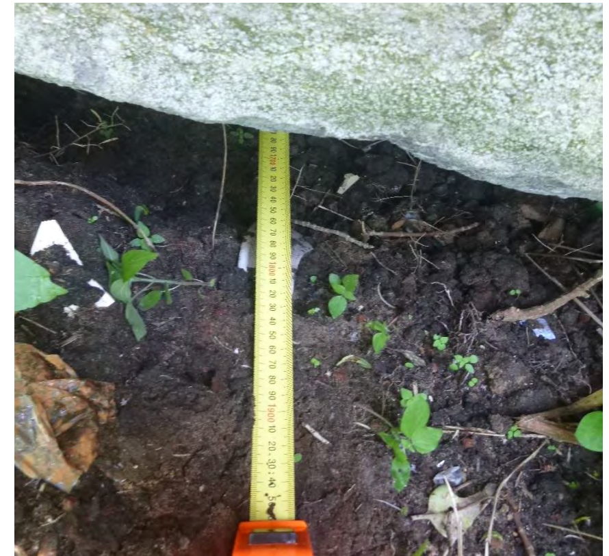
Photo 5. To north of Section 3 showing 1900mm penetration of tape measure into void/weathered seam.
