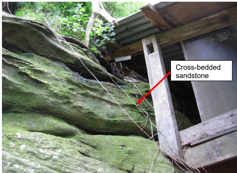
Mapping Traverse 103, Photo 3 – Oblique view of mapping traverse 103 from below, with cross--bedded sandstone exposed, as shown.
