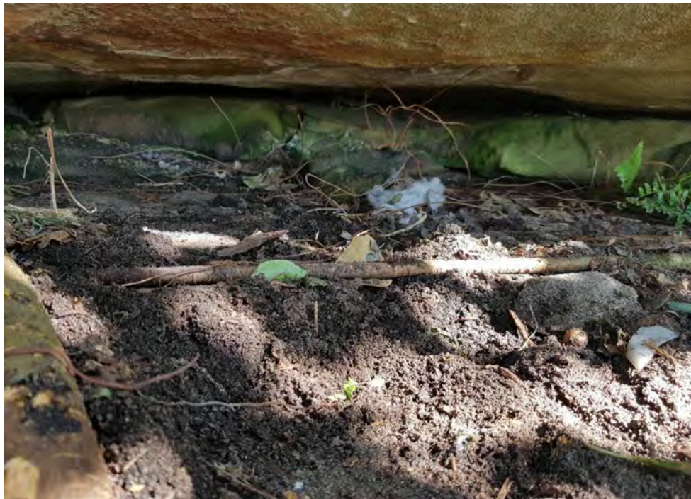
Mapping Traverse 105, Photo 1 – View within a cave formed below a bed of massive sandstone, along a bedding parting defect. Depth of cave from front face is 1.2 m, with sandy colluvium on floor of cave.
