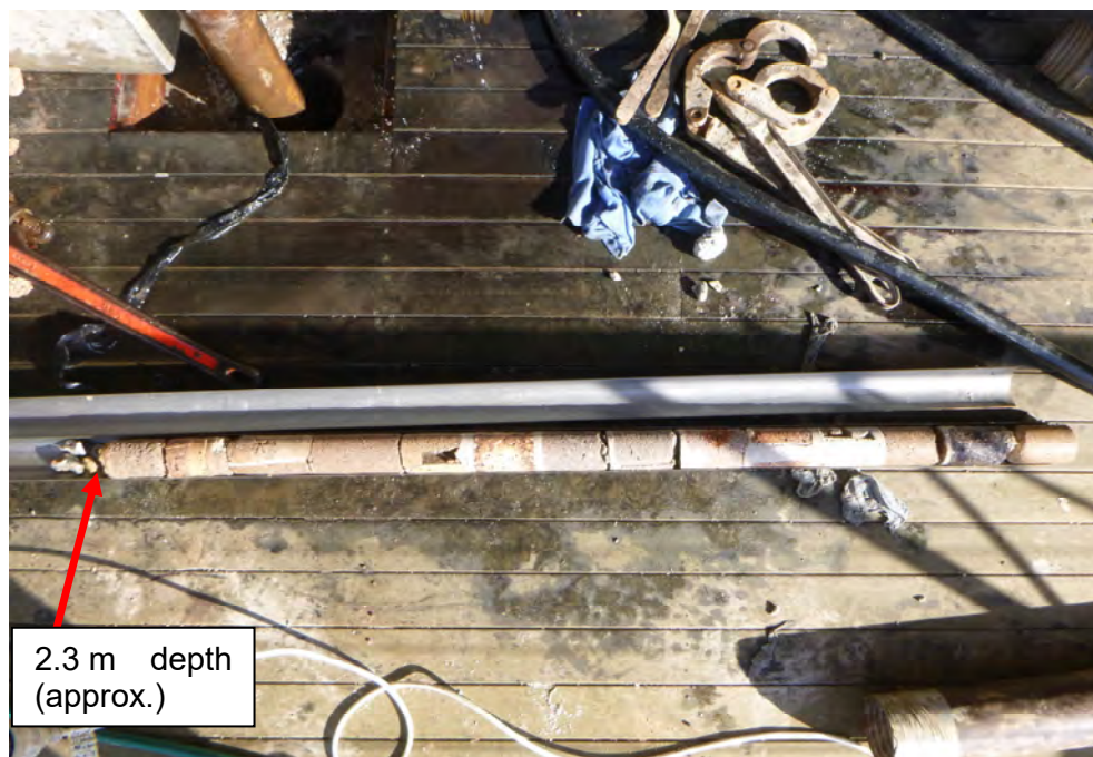
Photo D2 – View of mortared bricks within Borehole BH202. The start / top of the bricks is indicated as shown (approximate start / top depth of 2.3 m).
