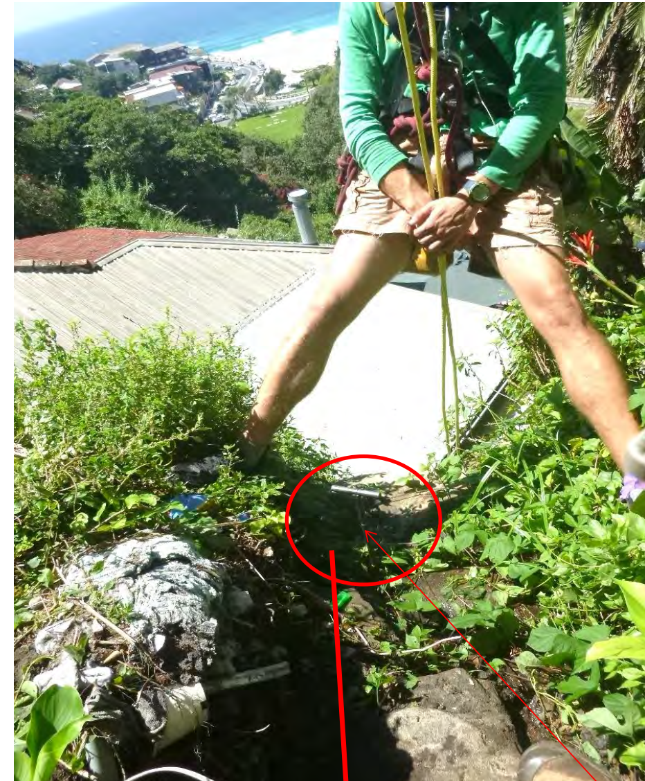
Photo 8. Outer edge of Section 3. Note 1m long steel test probe inserted 700mm into an open, though sand filled, joint, approximately 700mm back from the cliff crest.
