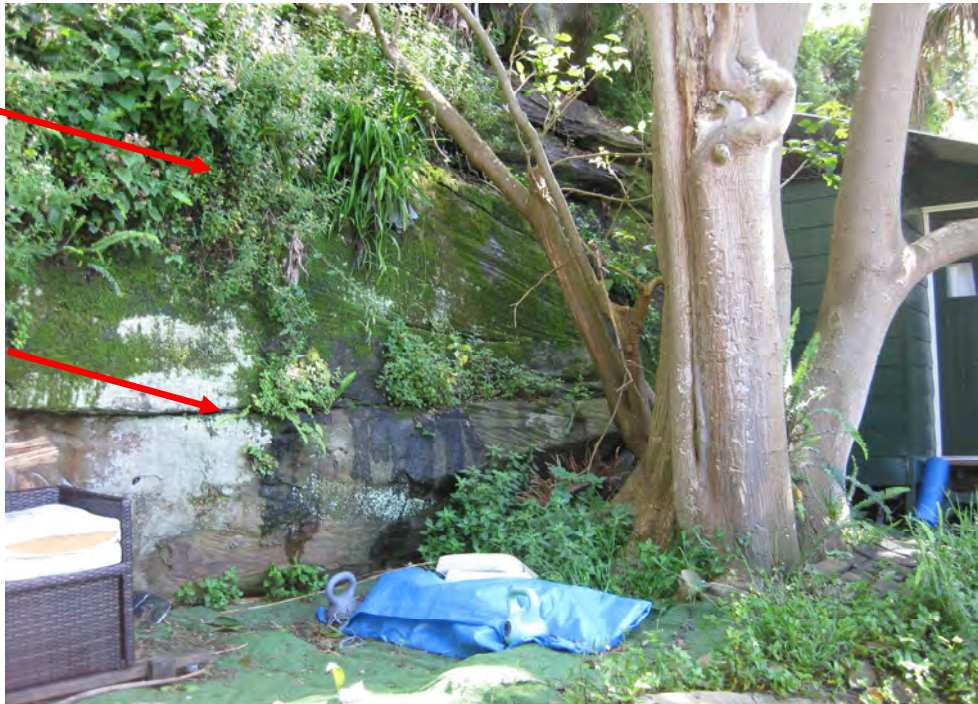
Mapping Traverse 104, Photo 3 – View north of mapping traverse 104. Continuous bedding planes within cross-bedded sandstone are indicated as shown.
