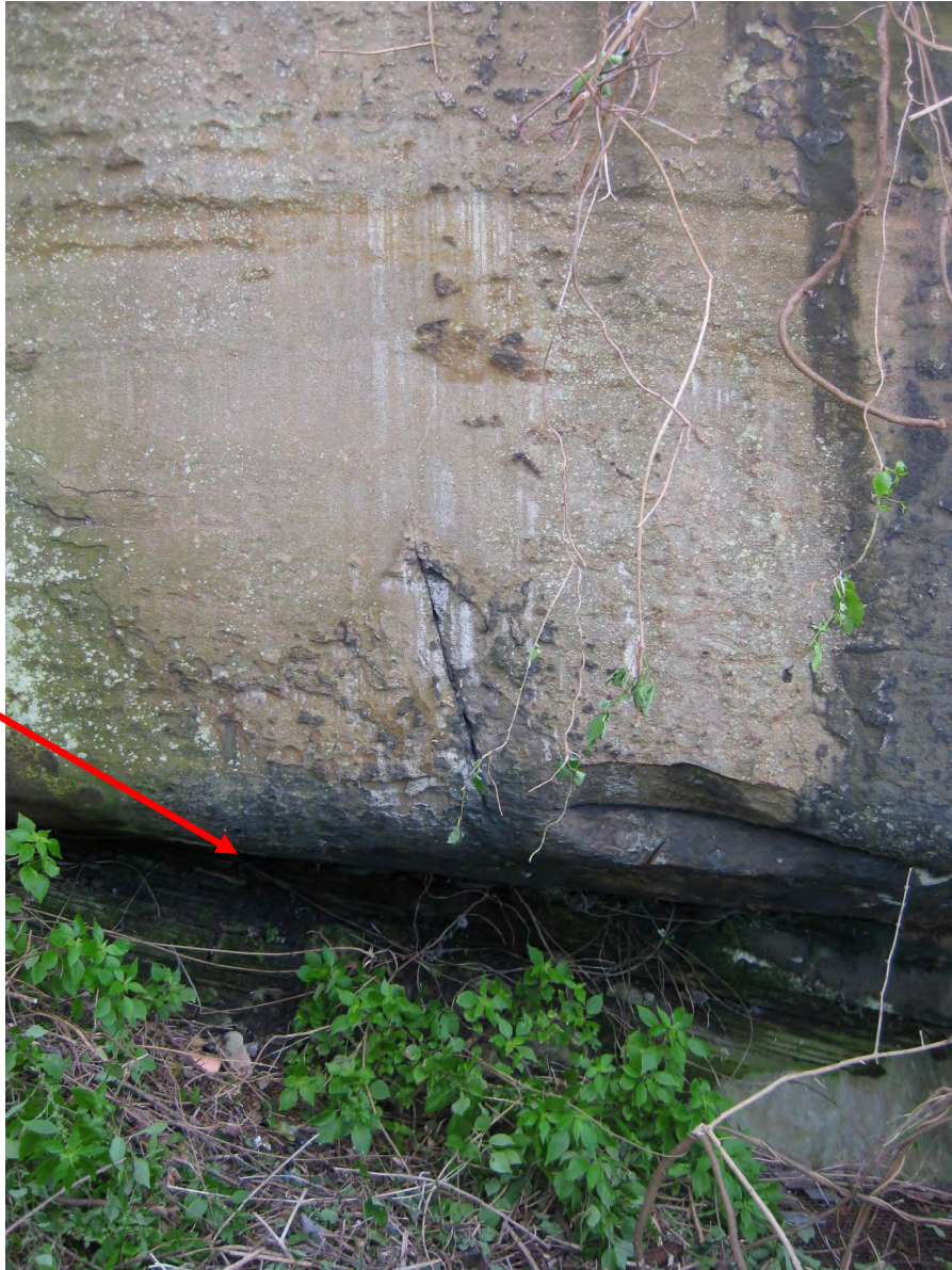
Mapping Traverse 108, Photo 3 – View of lower part of slope along mapping traverse 108, below Photo 2. Overhang formed on continuous bedding parting defect, indicated as shown.
